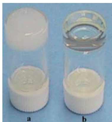
Figure 1. Two aqueous gels composed of 2 (0.2 wt %) (left) and 4 (0.05 wt %) (right), which are stable when inverted as shown.
